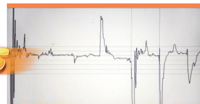
Traditional wave-reflect location: impulse current method
